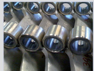
Hastalloy-wings with shrink-fitted TC-bearings
